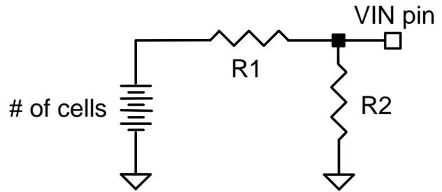
**Figure 13: Resistor divider network at the VIN pin**
