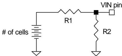
Figure 11: Resistor divider network at the VIN pin
